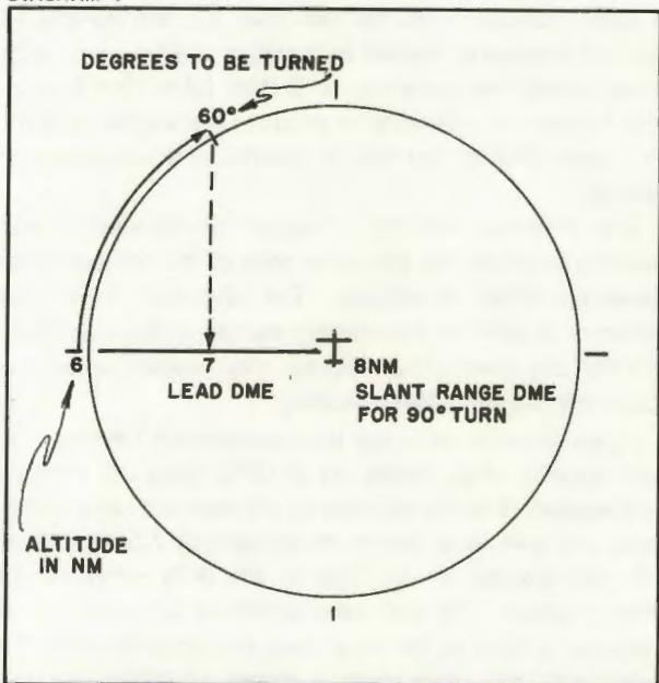
SLANT RANGE LEAD POINT FOR TURNS OTHER THAN 90 DEGREES
