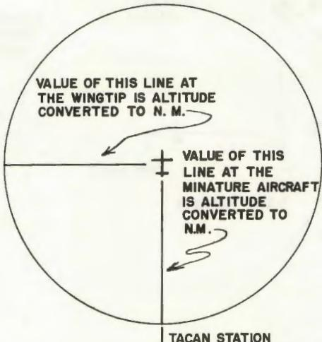
SLANT RANGE LEAD POINT FOR A TURN OF 90 DEGREES
