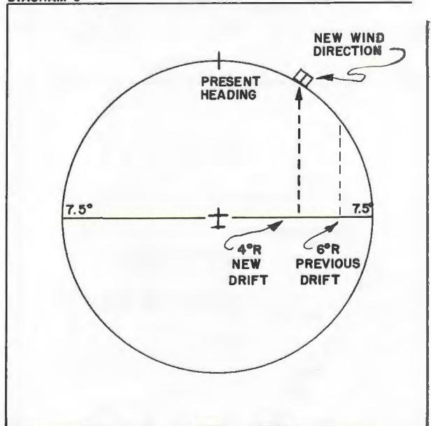
DETERMINING THE NEW WIND DIRECTION
