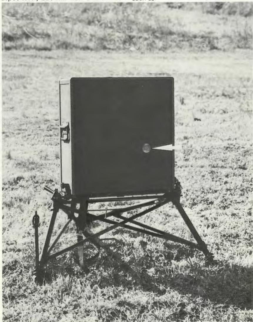
The complete TALAR transmitter weighs only 50 pounds making it highly transportable and requires only about five minutes to set up. Note the borescope sight used for establishing the glide path.
