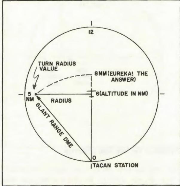
SLANT RANGE LEAD POINT FOR A TURN OF 90 DEGREES WITH THE VALUES IN POSITION
